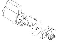
Remove Cylinder Cap, Tailpiece, Pin, and Spring
